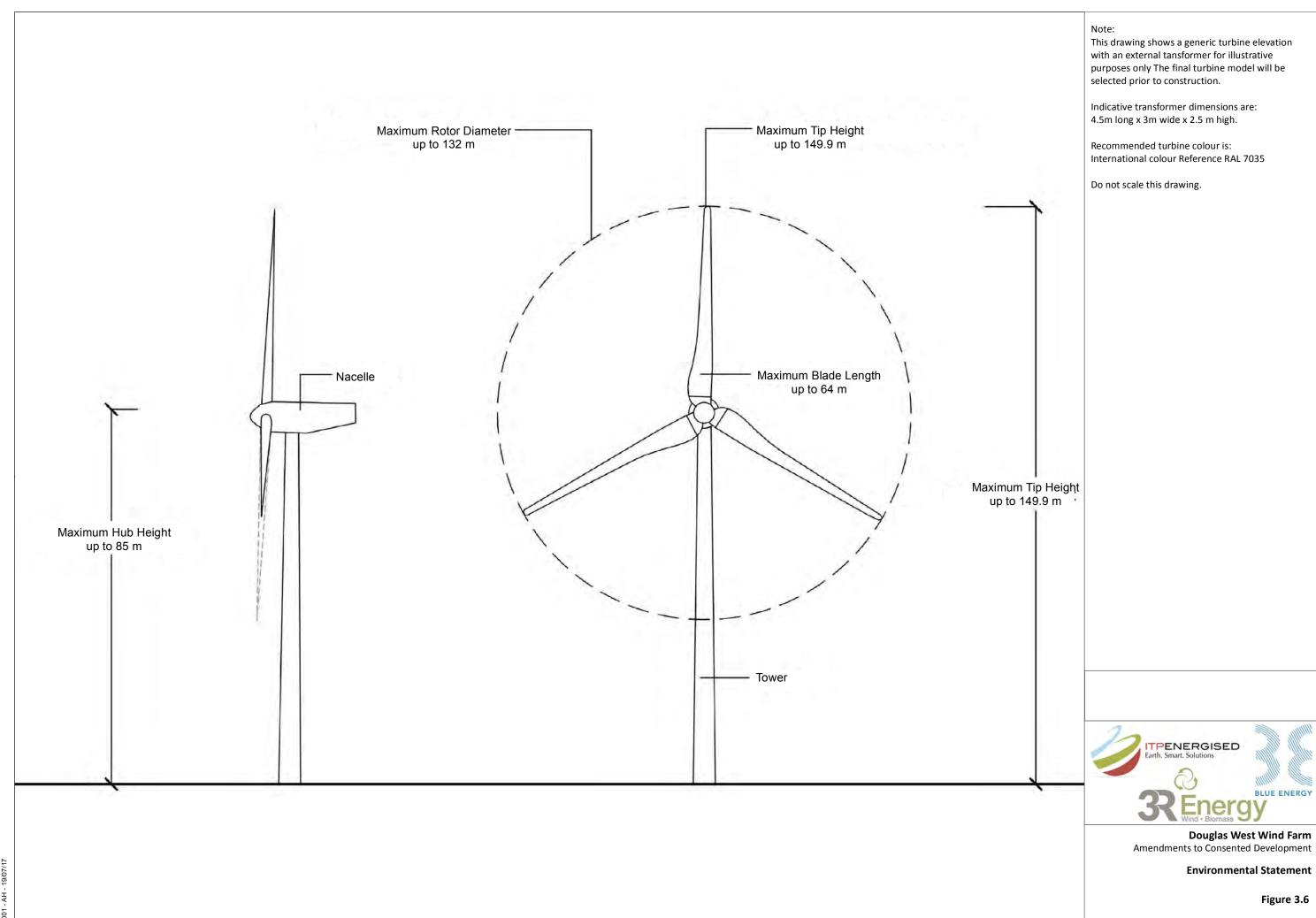
**Typical Turbine Elevation Drawing**
